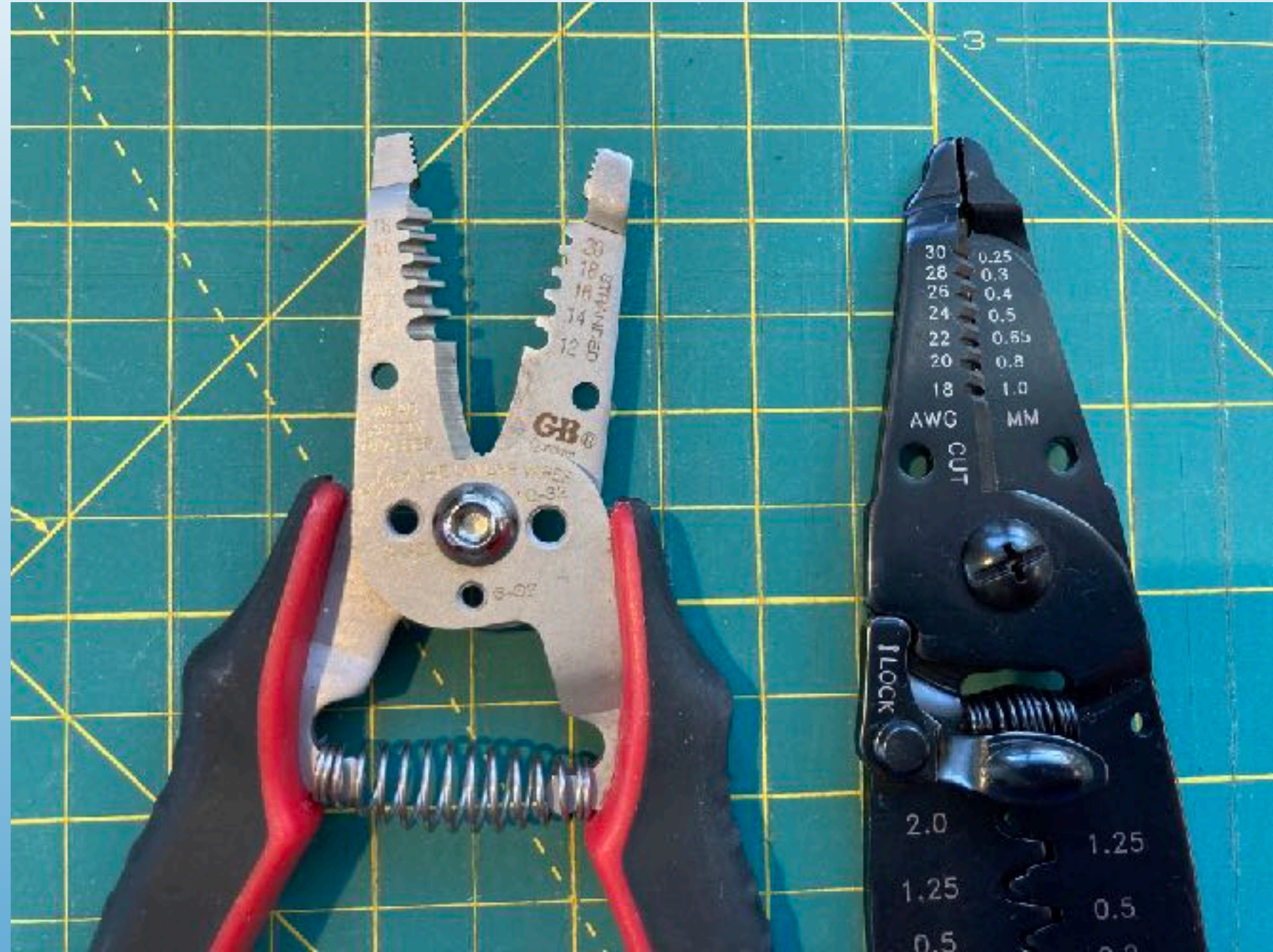
Wire strippers have different slots for various gauges of wire.
